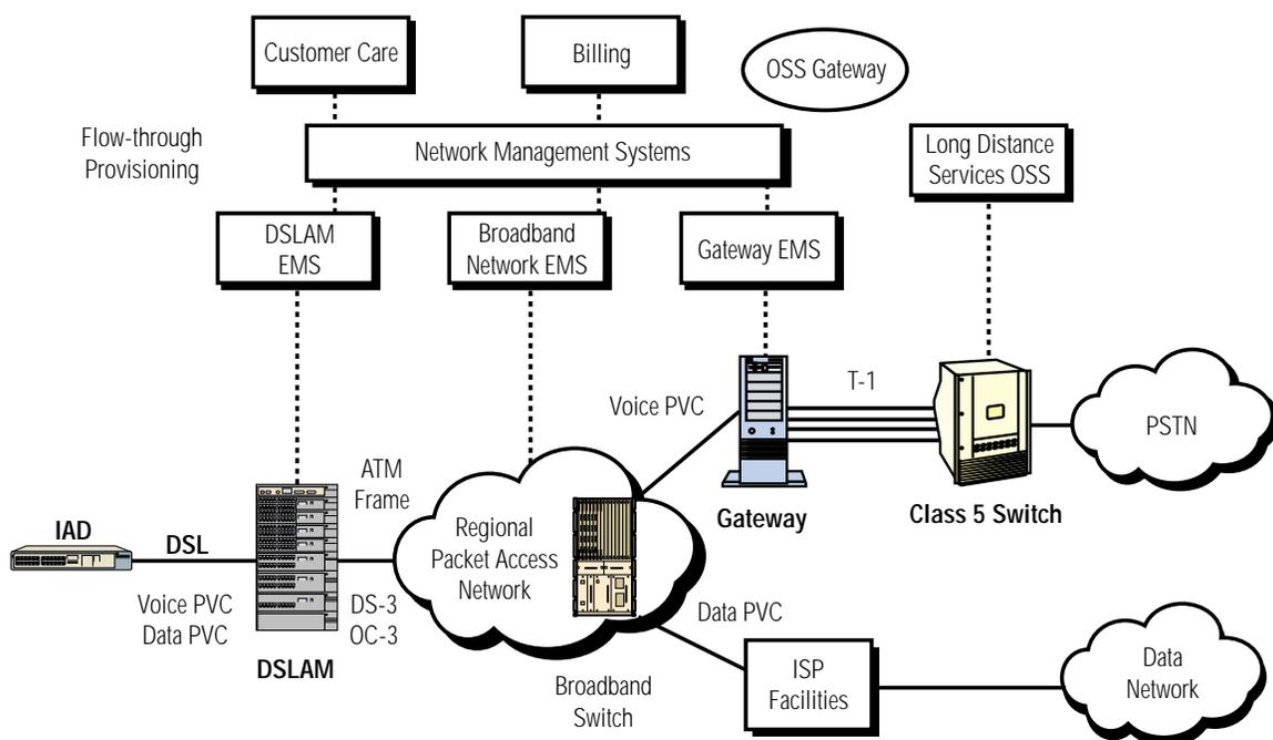
Figure IV-2 shows Tollbridge's IP local architecture for voice over DSL using the media gateway control protocol (MGCP) and Session Initiation Protocol (SIP) for call control.
